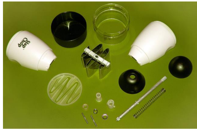
FIGURE 4 TEAM 20, FAZAAD ALLY, EVAN MCARTHUR AND JONATHAN SWEET “SLAP CHOP,” DISASSEMBLED PARTS, FALL 2012
