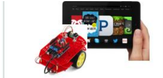
FIGURE 6. An Android (Kindle Fire) and a microcontroller bot communicating via the Bluetooth channel.
