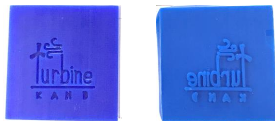
FIGURE 2 AN EXAMPLE PRODUCT FROM THE TEAM LOGO PROJECT. (LEFT) THE WAX MOLD THAT IS CNC MACHINED, (RIGHT) THE CAST SILICONE STAMP.
