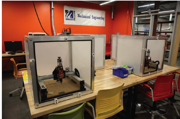
FIGURE 1 THE PROTOTYPING AND CNC BAY IN THE UNIVERSITY OF MASSACHUSETTS LOWELL MAKERSPACE. EACH PICTURED ENCLOSURE CONTAINS A SHAPEOKO II CNC MACHINE.
